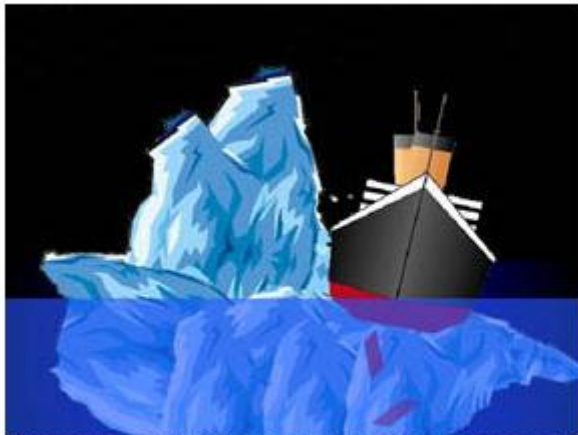
Ships tremendous weight bearing down on ice shelf, levering the above water portion of the berg toward its starboard side. The resulting brush depositing chunks of ice on the forward well deck.
